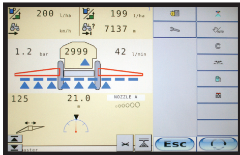
3_According to the assigned key, the product is released from the predefined sections
