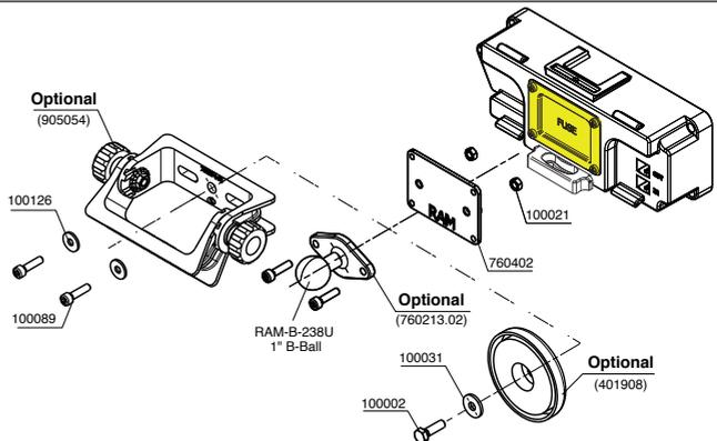
the FUSE cover, using the RAM support kit 906452 (order separately Fig.4) with:
