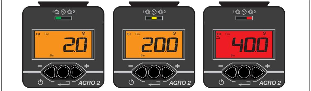
The full scale value of the transducer is chosen. The set values are: 10 - 16 - 25 - 60 - 100 - 200 - 250 - 400 - 600 - 1000 - 1500 BAR.
